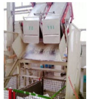
Discharging of containers with a comb lift
