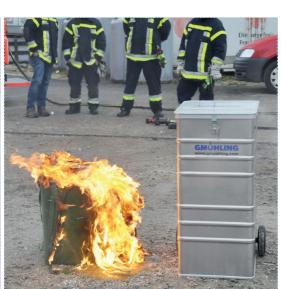
The data disposal container successfully completed the test, only a little soot was visible.
