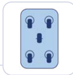
Wheel arrangement E: 4 swivel castors, 2 with wheel brakes and 1 fixed castor
