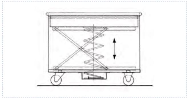
**Trolley with spring-loaded bottom D 04 based on pantographic system, aluminium & anodised**
