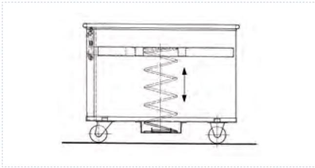
**Trolley with spring-loaded bottom D 1408 and D 5408 with sliding guidance, aluminium & anodised**
